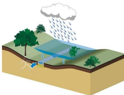
Noue infiltrante (Source : Architecture & Climat)
